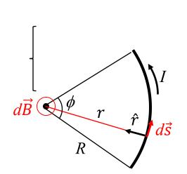
Calculate the  $\vec{B}$ -field the center of a circular arc spanning an angle  $\phi$  and of radius R carrying a steady current I.
