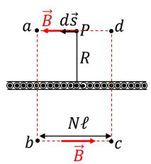
The  $\vec{B}$  -field is either paralle or perpendicular to the  $d\vec{s}$  steps.
