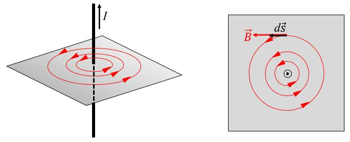
It has been found that the product of the component of  $\vec{B}$  along a small step  $d\vec{s}$  summed around a closed contour enclosing a current equals that enclosed current times the permeability constant. That is,  $\oint \vec{B} \cdot d\vec{s} = \mu_0 I_{enc}$ . This is Ampere's law.
