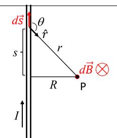
Calculate the  $\vec{B}$ -field a distance R from a long straight wire carrying a steady current I.
