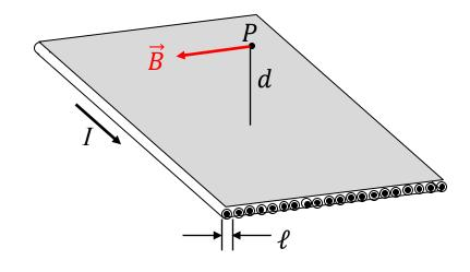
Recall that by symmetry, the  $\vec{B}$ -field at *any point* above the sheet to directed to the left. Using a similar argument, the  $\vec{B}$ -field below the sheet is directed to the the right.
