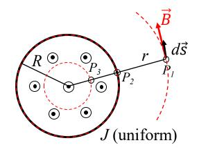
As in the previous example,  $\vec{B}$  and  $d\vec{s}$  are parallel and that  $|\vec{B}|$  is a constant at any point on a given field line. Choosing a circular Amperian loop,
