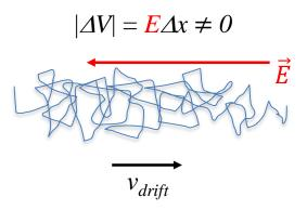
Note that  $v_{drift}$  is opposite to the electric field since the charge carriers (electrons) are negative (q = -e).
