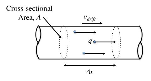
The amount of charge  $\Delta q$  in the volume  $A\Delta x$  is  $\Delta q = qn(A\Delta x) = qnAv_{drift}\Delta t,$
