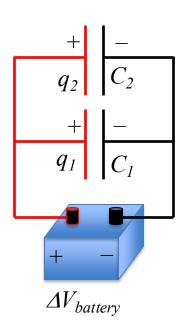
The battery transfers electrons from the left plates to the right plates. Note that each capacitor has the same  $\Delta V_{battery}$  across them.
