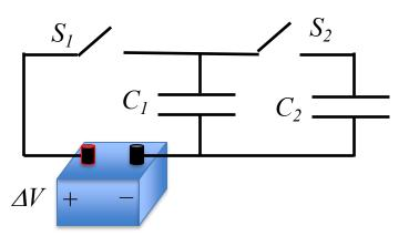
When  $S_1$  is closed,  $C_1$  acquires a charge  $q_{1i} = C_1 \Delta V$ .
