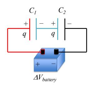
The battery transfers electrons from the left plate of  $C_1$  and the right plate of  $C_2$ .
