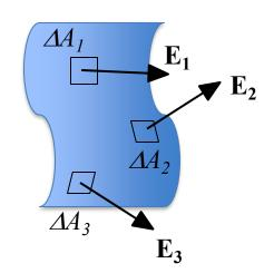
In this case, the electric flux through the surface by summing over all the  $\Delta A$ 's where each  $\Delta A$  is small enough to consider the **E**-field through that  $\Delta A$  to be constant. Then,
