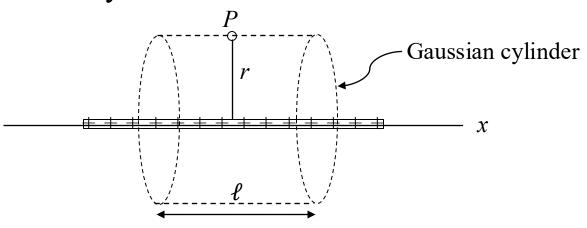
$$\Phi_E = \oint \vec{E} \cdot d\vec{A} = \int_{\text{left cap}} + \int_{\text{right cap}} + \int_{\text{cyl body}}$$
