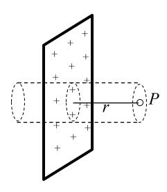
$$\Phi_E = \oint \vec{E} \cdot d\vec{A} = \int_{\text{left cap}} + \int_{\text{right cap}} + \int_{\text{cyl body}}$$
