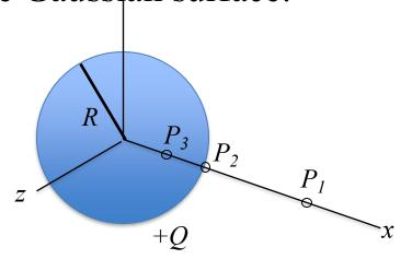
Note that  $\vec{E}$  and  $d\vec{A}$  are parallel at all points on the chosen Gaussian surface regardless of the value of r.
