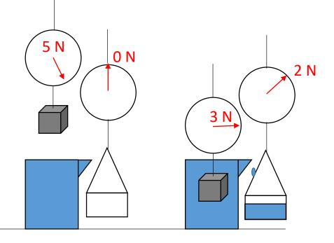
Note that a fully submerged object displaces a *volume* of fluid equal to its own volume.
