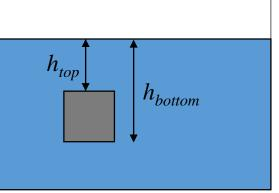
the same. Therefore, the downward force acting on the top face has a smaller magnitude than the magnitude of the upward force acting on the bottom face. As a result, the water Exerts a net upward force (called the buoyant force) on the cube.
