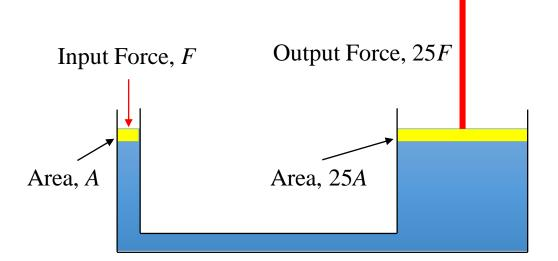
Consider the U-shaped container fitted with (assumed frictionless) pistons where one side has a larger area than the other. A small weight placed on the small piston produces an additional pressure on that area. This change in pressure is transmitted undiminished to all part of the fluid and to the large piston. With the same pressure on the larger piston, the force on the larger piston must be greater. So, the small force is amplified to lift the heavy load.
