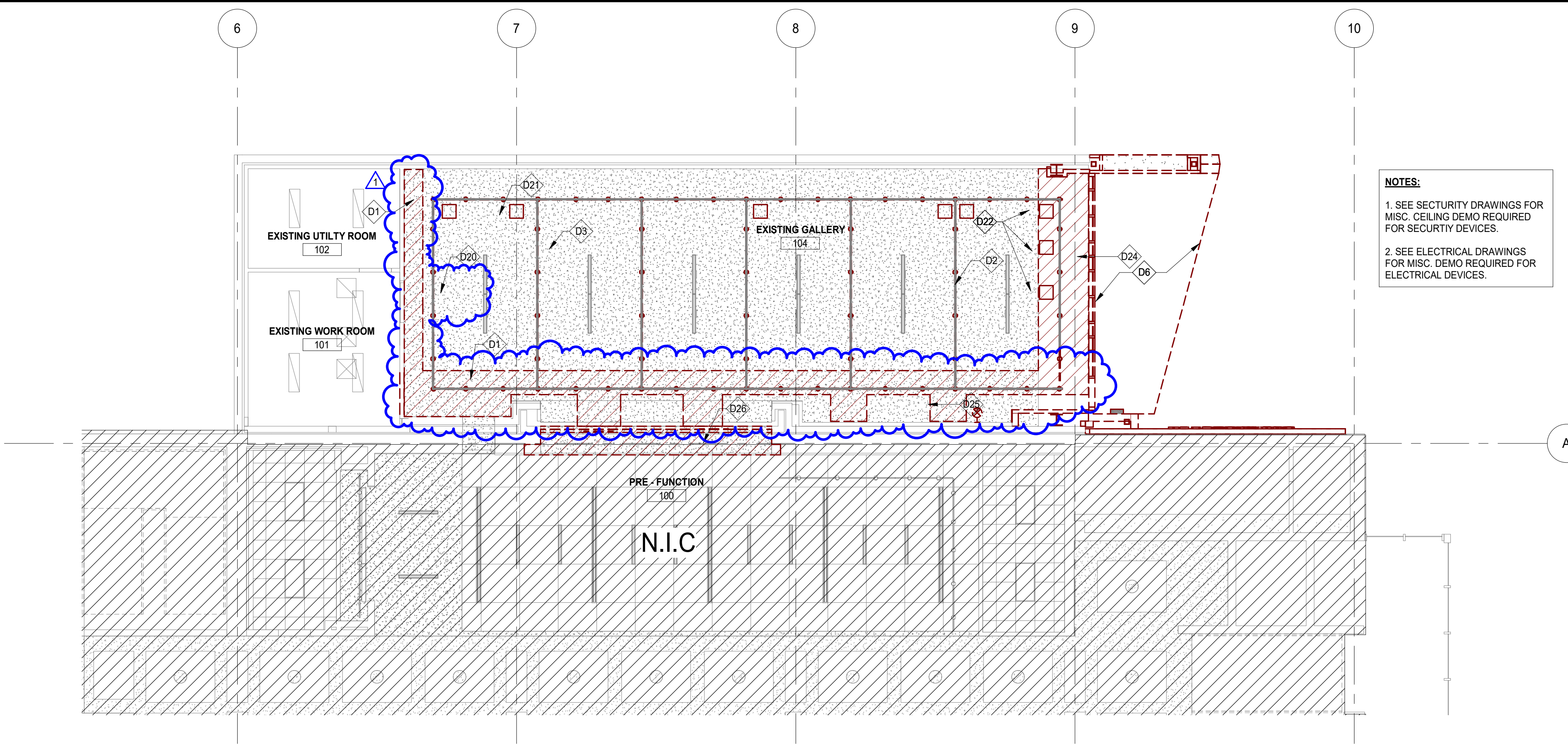
2 DEMOLITION REFLECTED CEILING PLAN SCALE: 1/8" = 1'-0"
